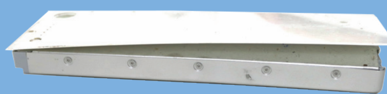
Case appears cracked due to unseen bloated cells
