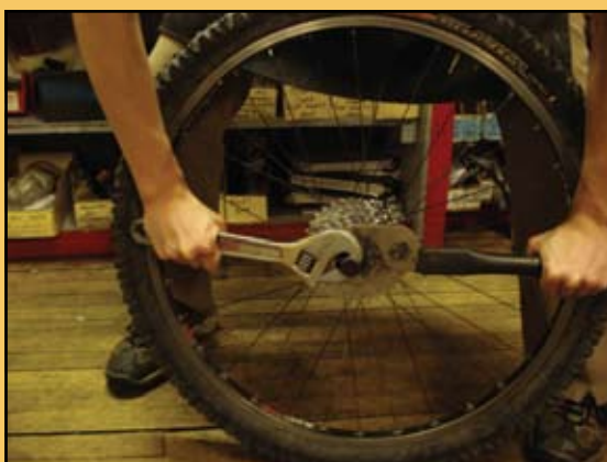
Double push down technique for removing cassette Lock ring
