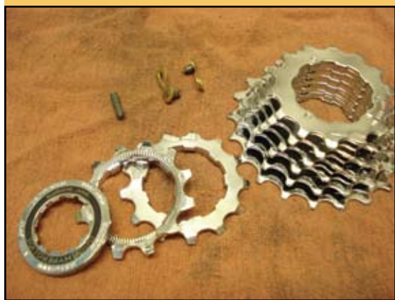
(Top) Shimano chain pin, SRAM Power Link (bottom) Cassette with two cogs and lock ring
