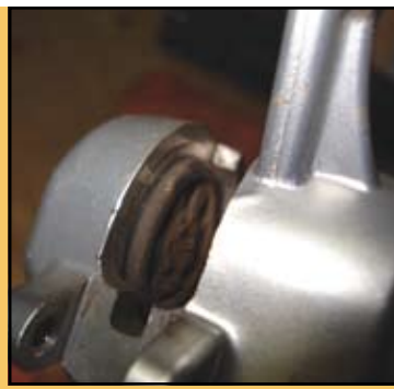
Brake Piston in the 'Out' position.
