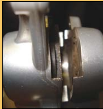
Brake Piston in the 'In' position.
