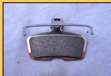
Place the spring between the pads and across the pad material prior to installation. Photo by Tom Jow
