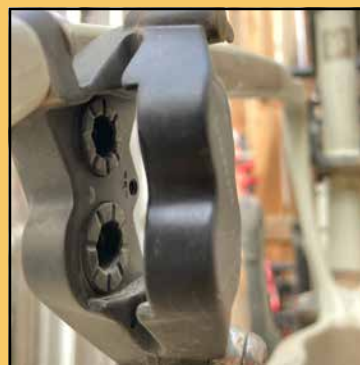
Clean inside the caliper prior to pad installation. Photo by Tom Jow
