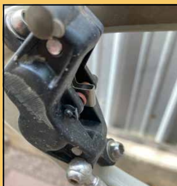
Be careful removing the pin clip. They are small and get lost easily. Photo by Tom Jow
