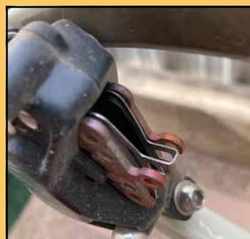
Push or pull the old pads out from the top of the caliper. Installation of the new pads happens opposite of removal. Photo by Tom Jow
