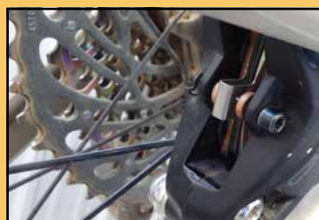
The brake pad safety pin is a small diameter and requires little torque to tighten. Photo by Tom Jow
