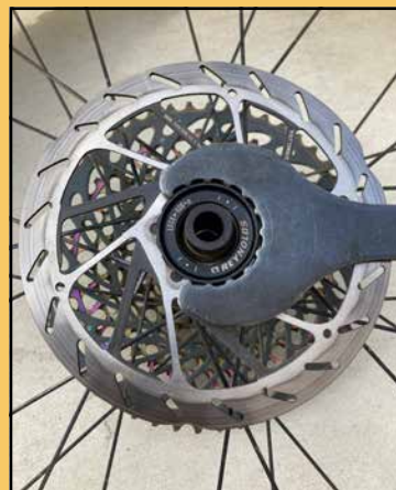
If you need to remove the rotor: Use a Shimano bottom bracket tool to remove the Centerlock locking. Be gentle on installation. It is easy to cross thread at the start. Photo by Tom Jow
