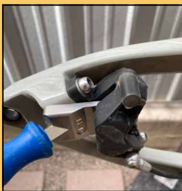
Use a Park PP-1 or similar tool to press the pistons back into their bores before removing the old pads. Photo by Tom Jow
