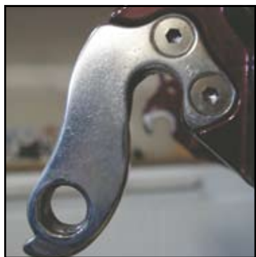
Above: A typical rear derailleur hanger with two bolts.
